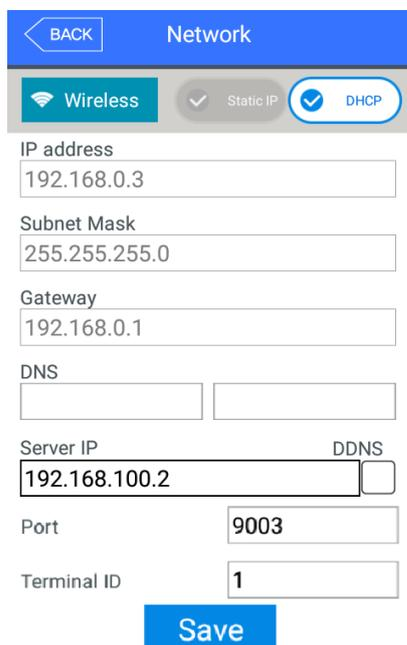
When the Wi-Fi dongle is connected to the USB port on backward of the UBio-X Pro2 device, this icon [Wireless] will be come up automatically on the Network screen as same as left picture.
