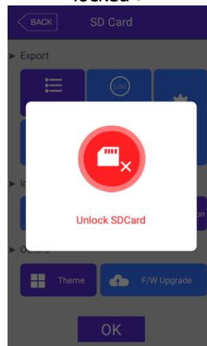
※ It works only if the SD Card is inserted, and it should be inserted with the back side face forward like the figure. (The size of the SD Card should not exceed 32G.)
